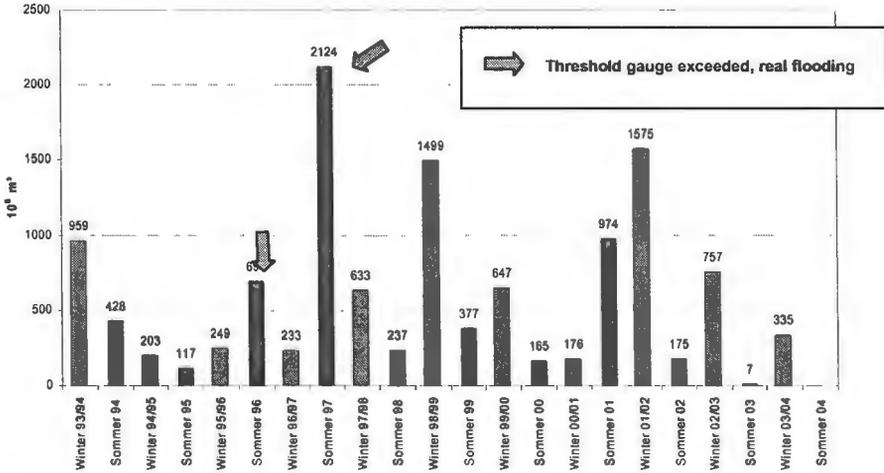
**Figure 10.** Water volume flowing through Polder A/B during the course of a decade. Winter flooding: November – April; (hypothetical/real) Summer flooding: April – November.
