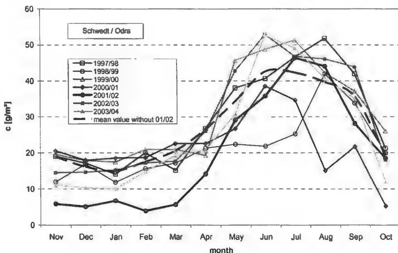
**Figure 4.** Concentration of suspended sediments (dry weight) in the Lower Odra River at polder inflow. Dotted line shows a mean value of all indicated years except the year 2001/2002 with an outstanding low sediment concentration (thick line).
