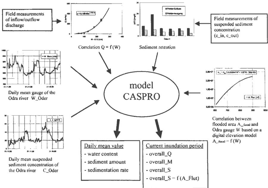
**Figure 2.** Input and Output parameters included in the CASPRO model.
