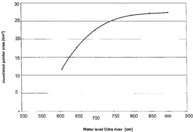
**Figure 6.** Correlation between flooded polder area and Odra gauge based on a digital elevation model
