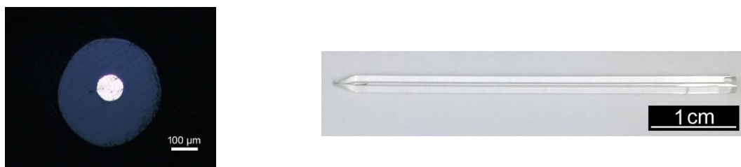
Fig.10.1. Micrographs of the Au microelectrode. Left image shows front view, right image – side view.
