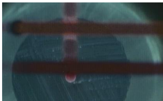
Fig. 10.22. Optical micrograph presenting local electrodeposition of CuNS on predeposited AuNS on the ITO substrate.
