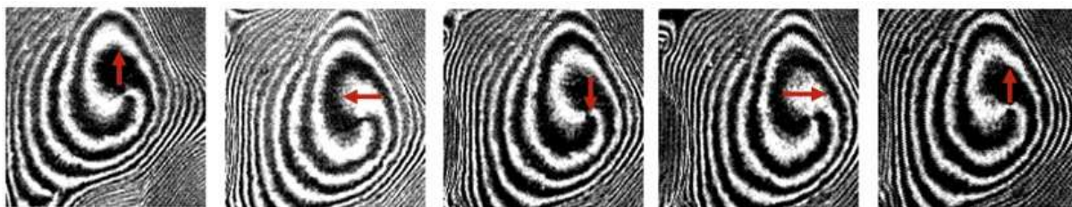
Figure 28 Sequence of the images taken with time delay 6 s indicating the changes of the tilt azimuth
