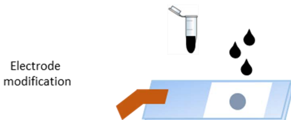
Figure 5.3.3.3 Schematic electrode surface modification.
