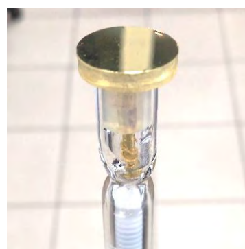
Figure 2.1-1. Single-crystal Au(111) electrode in a glass capillary.
