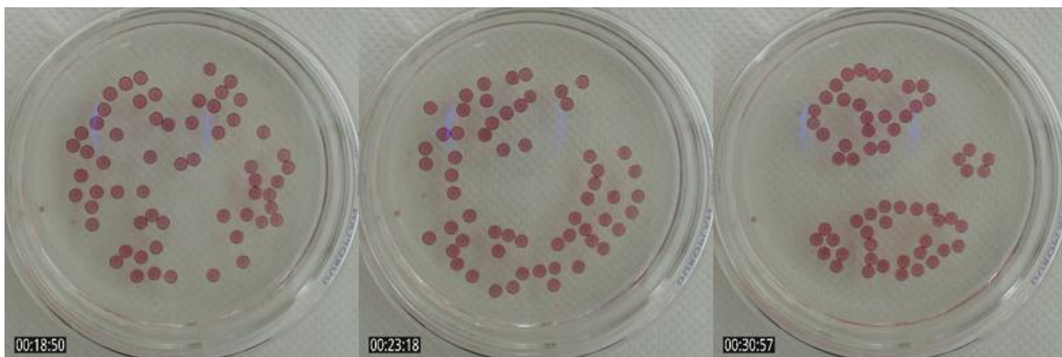
Figure IV.19: Behavior during Stage II. The droplets are beginning to loosely associate in clusters. Snapshots taken at times 18m50s, 23m18s and 30m57s as seen from left to right. Full time interval is 11minutes.
