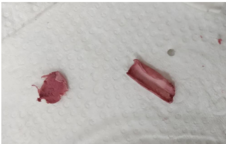
Figure III.13: Remnants of objects made from camphor-camphene wax that was stored and reheated inside polypropylene falcon tubes and left exposed to an open atmosphere.
