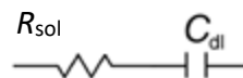
Figure 2-13. The equivalent circuit with a non-faradaic electrochemical process for the (non-conducting polymer film)-coated electrode in a supporting electrolyte solution.
