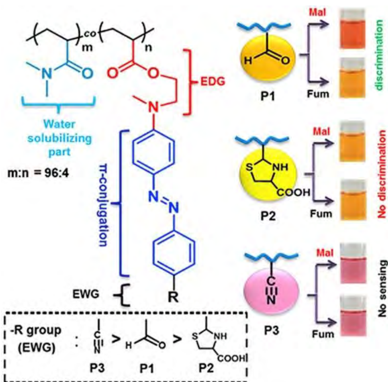
Figure 69. Structures of a series of water-soluble polymers 65(P1) , 66(P2) and 67(P3) and their efficiency in the colorimetric discrimination of maleic (Mal) and fumaric (Fum) acids.
