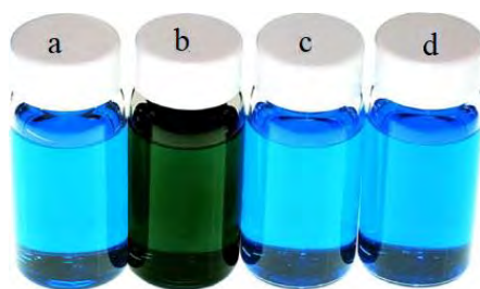
Figure 3. Effect of phthalate isomers on color changes of 1 : (a) 1 ; (b) 1 +phthalate; (c) 1 +isophthalate; (d) 1 +terephthalate. Adapted with permission from the Elsevier. Copyright 2006. 5
