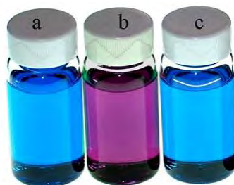
Figure 61. Photographs of the solutions: (a) 2 ; (b) 2 +maleate; (c) 2 +fumarate. Adapted with permission from the Elsevier. Copyright 2006. 5
