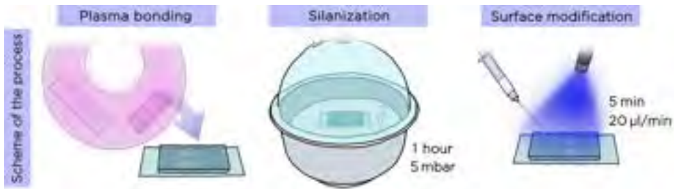
Figure 4.1: Scheme of hydrophilic surface modification: following standard plasma bonding of the chip, we depose vapours of Silane on the surface, positioning the chip in a vacuum chamber with 30 \mu\text{l} of Vinyltrichlorosilane for 1 hour. Finally, we flush the GelMA solution inside the channels while using UV light to promote the bonding between GelMA polymers and the Vinyltrichlorosilane.
