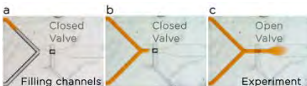
Figure 2.7: Preliminary measures introducing a red ink within a previous chip design. (a) Flushing the red solution through the side channels with the closed valve, (b) preparing for the experiment, and (c) opening the valve and flushing the die within the chamber.
