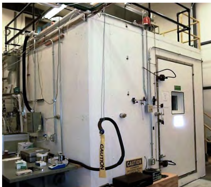
Figure 10. U.S. EPA indoor smog-chamber system, Research Triangle Park, North Carolina
