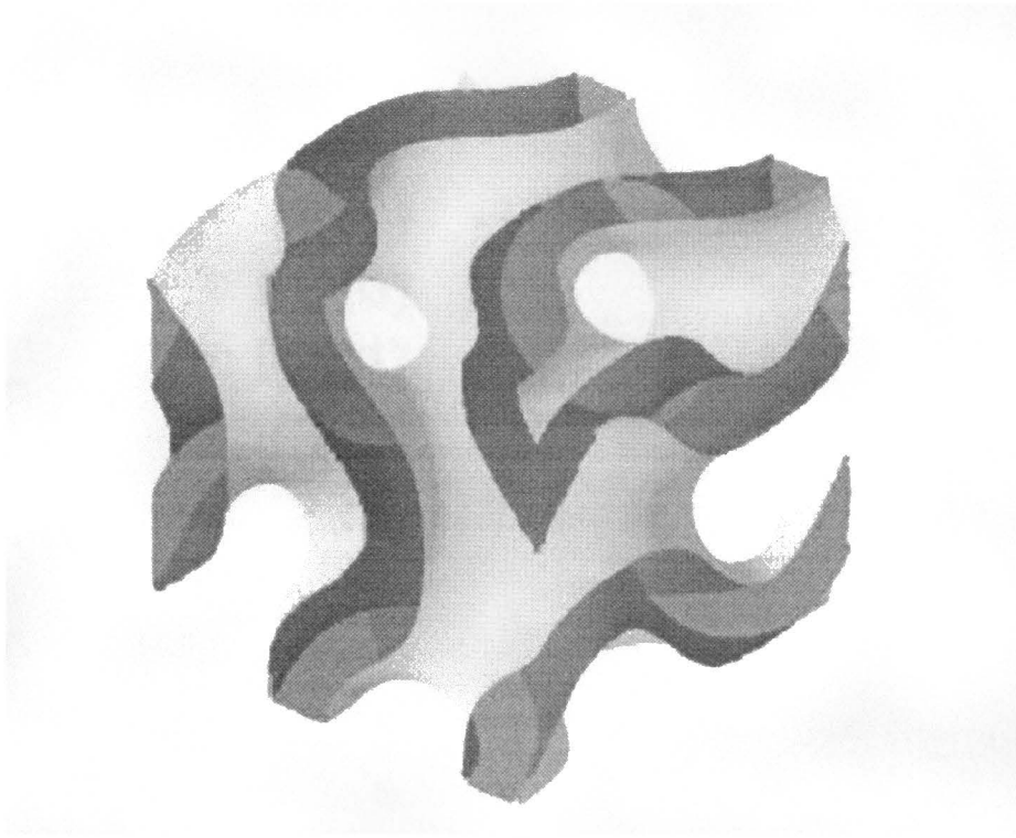
Figure 39: A computer visualization of the G gyroid TPS based cubic phase determined by fitting the experimental SAXS pattern (Figure 38). The darker areas correspond to the subvolume ( \phi = 0.45 ) occupied by the polymerized bilayer.
