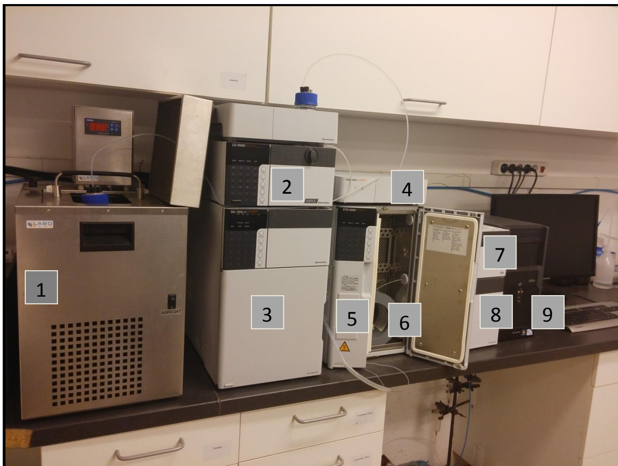
Figure 17. The experimental setup: 1- heating controller; 2- pump; 3- autosampler; 4- degasser unit; 5- thermostat; 6- capillary; 7- UV-Vis detector; 8- fluorescence detector; 9- computer.
