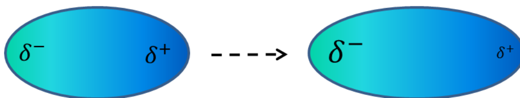
Figure 2. Dipole-induced dipole interactions. The electrons of the second molecule are attracted by the positive end of the first molecule. As a consequence, the electrons of the second molecule migrate to the left side and make the left side more negative.
