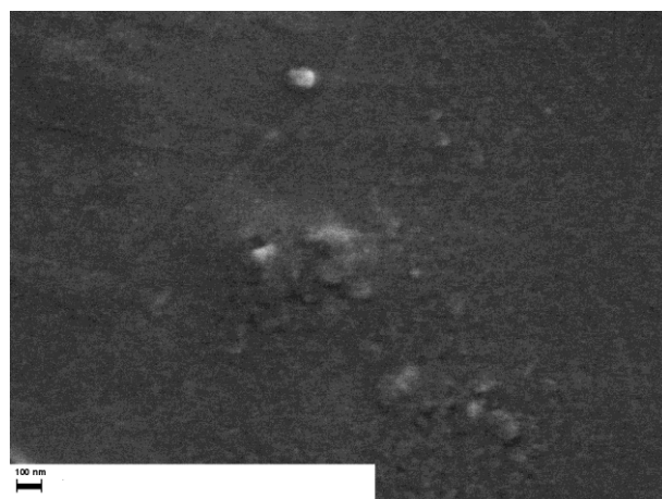
Fig. 15.1 SEM image of the ITO electrode coated with five CNPs-imidazolium functionalized silicate layers.
