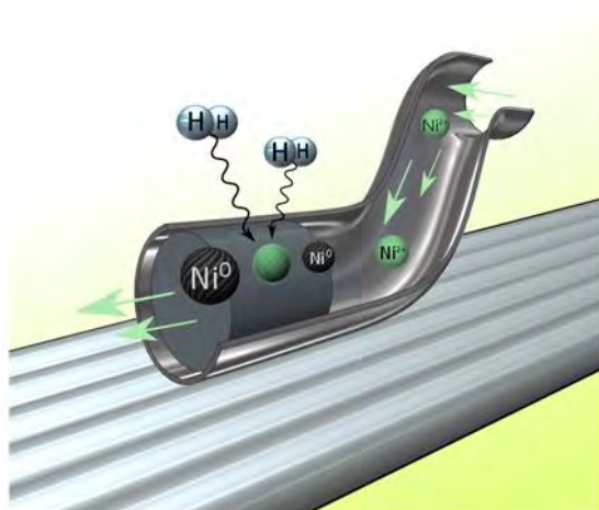
Scheme 8. On-the-fly catalyst accretion in continuous-flow micro-reactor.
