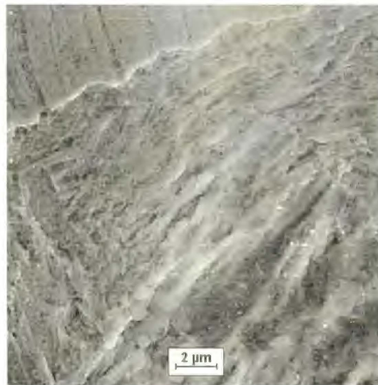
Figure 5.12. Appearance of the peeled-off ingress surface of the membrane subjected to high cathodic polarization. Steel 28I.
