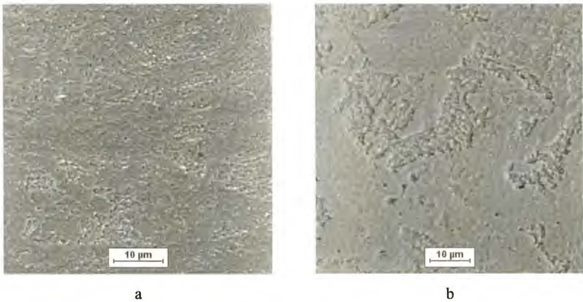
Figure 5.4. Change of the microstructure of subsurface layer of 25N steel due to the shot peening: a – shot peened layer; b- bulk material (SEM).
