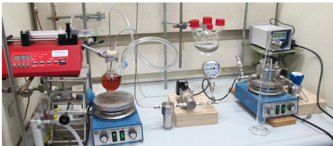
Figure 71. First version of the home-made continuous mini-plant designed and built in the group of prof. Vogt.
