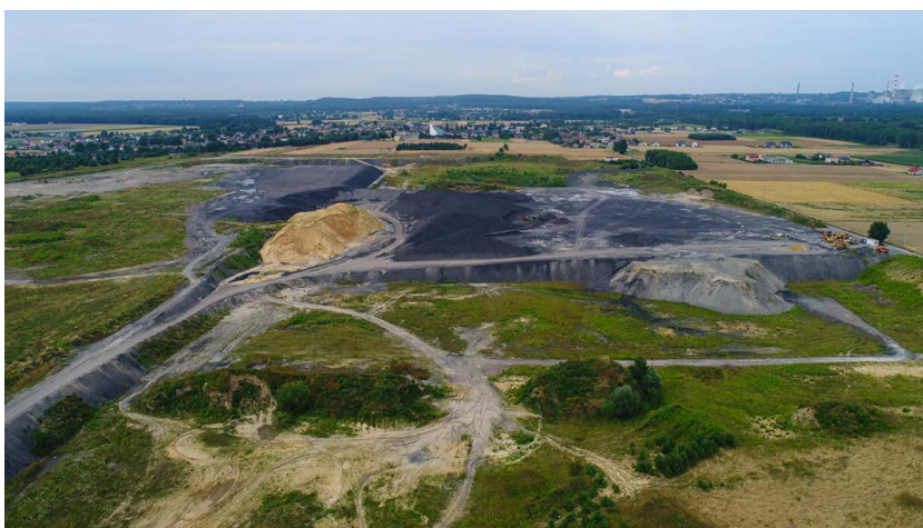
Figure 10. The area of the Gardawice sandpit (p. 3) reclaimed with mining waste. The excavation currently visible in front of the waste mass has been filled
