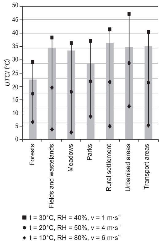
**Figure 4.** Average values for the *UTCI* under various types of land use and different weather conditions with a cloudless sky, and the difference between *UTCI* values for scenarios with an air temperature of 30°C or of 10°C (marked by grey bars).
