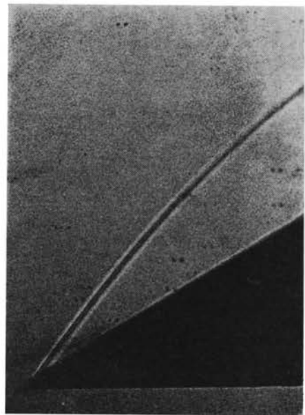
FIG. 11. Stationary oblique shock, M_S = 9.3 , \beta_K = 30^\circ , h_1 = 1 Torr, T_1 = 298 K.
