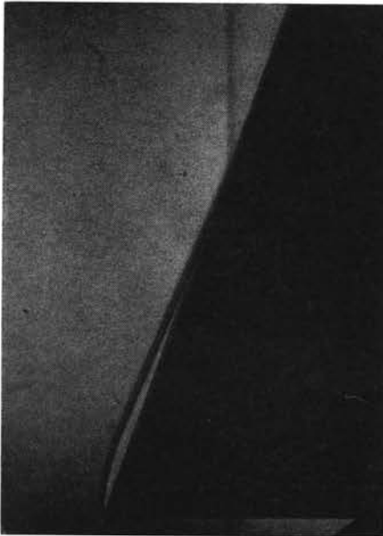
FIG. 10. Regular shock reflection, M_S = 9.2 , \beta_K = 70^\circ , p_1 = 1 Torr, T_1 = 295 K.
