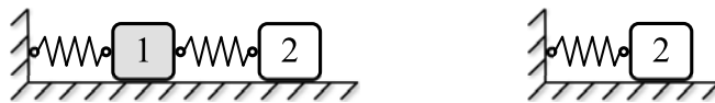
Figure 5.4. Numerical example of the 2-DOF mass-spring system: (left) the global system and (right) its isolated substructure.
