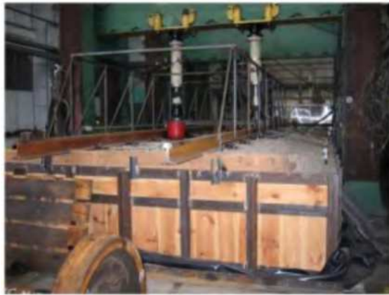
Figure 3.14. View of the testing stand for a new type of railway track [129].
