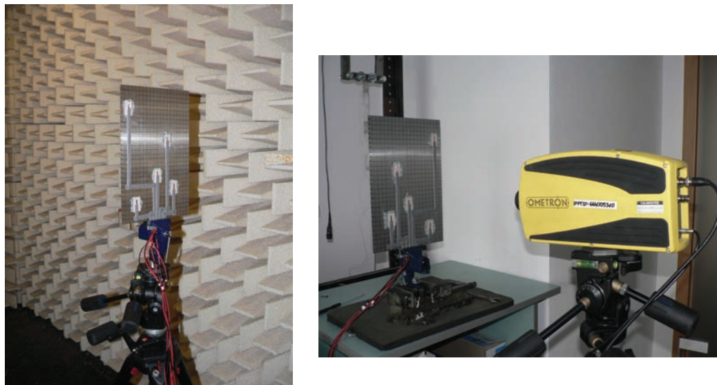
Figure 4.9. Thin aluminium plate with attached piezoelectric transducers in the laboratory stands used in the experimental investigations.
