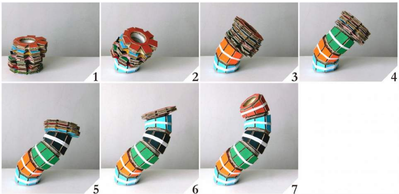
Figure 20. Deployment of a helical dPZ.
