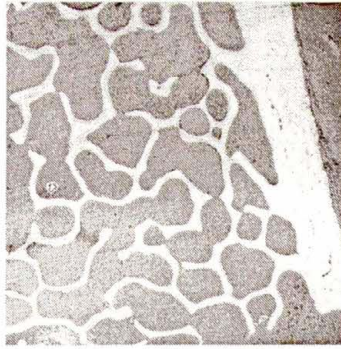
FIGURE 1. The acoustic microscope image of the trabecular structure of cancellous bone; frequency= 100 MHz, area= 3.2 mm×3.2 mm
