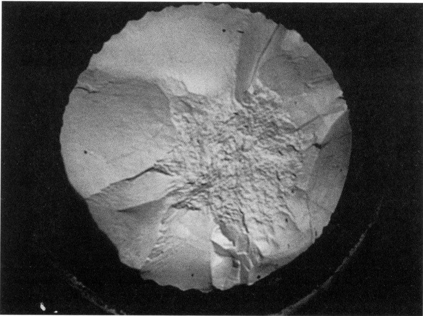
FIGURE 2. Image of the PAK A insulator fracture from the side of fixing device.
