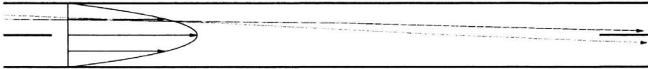
FIGURE 1.4. Schematic representation of the SPLITT Thin flow fractionation, or “SPLITT” cell. In a force field, say gravity, heavier particles move down faster and are separated in the lower exit whereas lighter particles leave through the upper exit.
