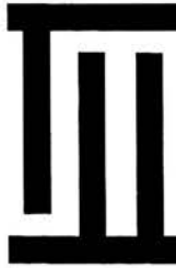
Figure 4.1: Three-finger-type IDT cell.
