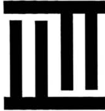
Figure 4.2: Double-electrode-type IDT cell.
