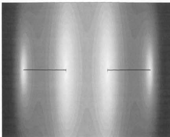
Figure A.2: Electric field for the case of two electrodes in vacuum (amplitude, logarithmic scale).
