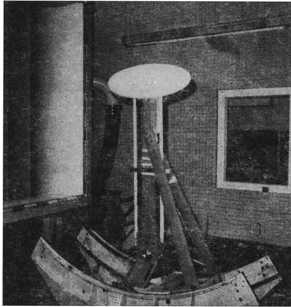
FIG. 2. Ellipsoid in the open test section of the 3m-low speed wind tunnel of the DFVLR Göttingen. Test set-up.
