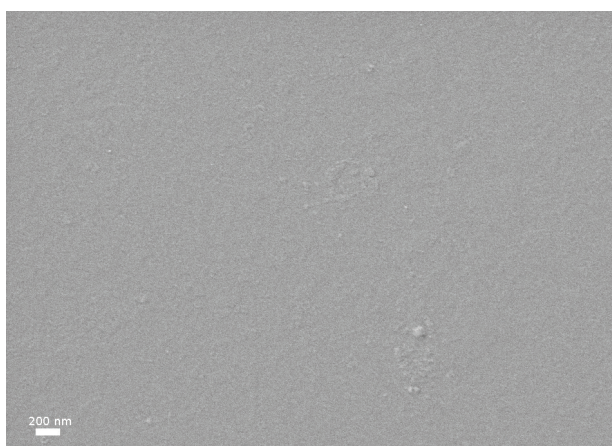
Fig. 13. SEM image of a glass slide with a 14 nm \text{AlN} layer after 177 deposition cycles. The surface has good uniformity with small ( \sim 10 nm) crystallites.
