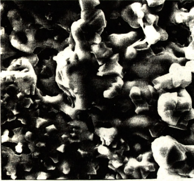
Fig.6 Surface microstructure of copper torn apart from alumina after bonding with CuO at 1348K (1075°C) SEM, x 2000.
