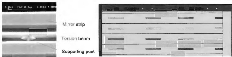
Fig. 7. Part of the mirror array in modified BESOI-technology.
